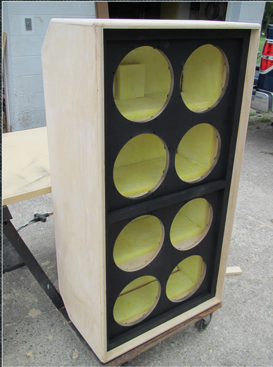
Here is the front of the cabinet sanded and ready to be covered.
