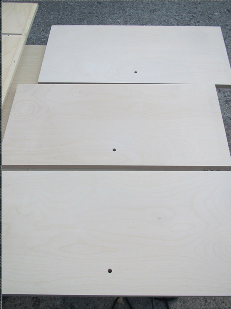
The divider pieces cut to size, with holes drilled for the speaker wires.
