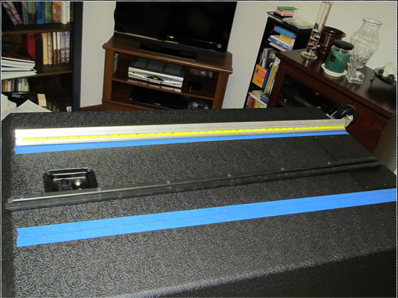
Laying out the mounting holes for the skid rails.
