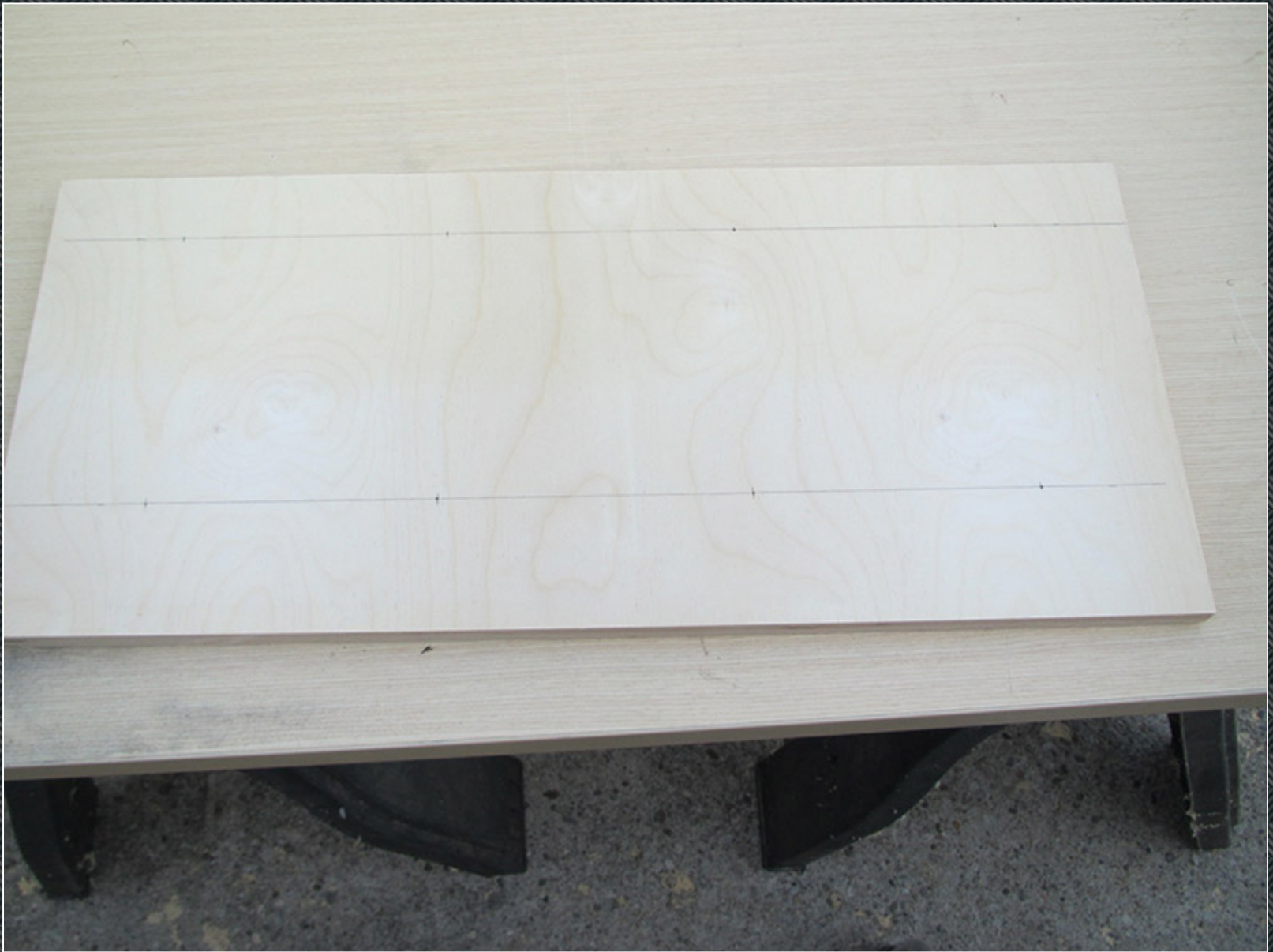
Here is the cabinet top piece laid out for the 8 foot cups.
