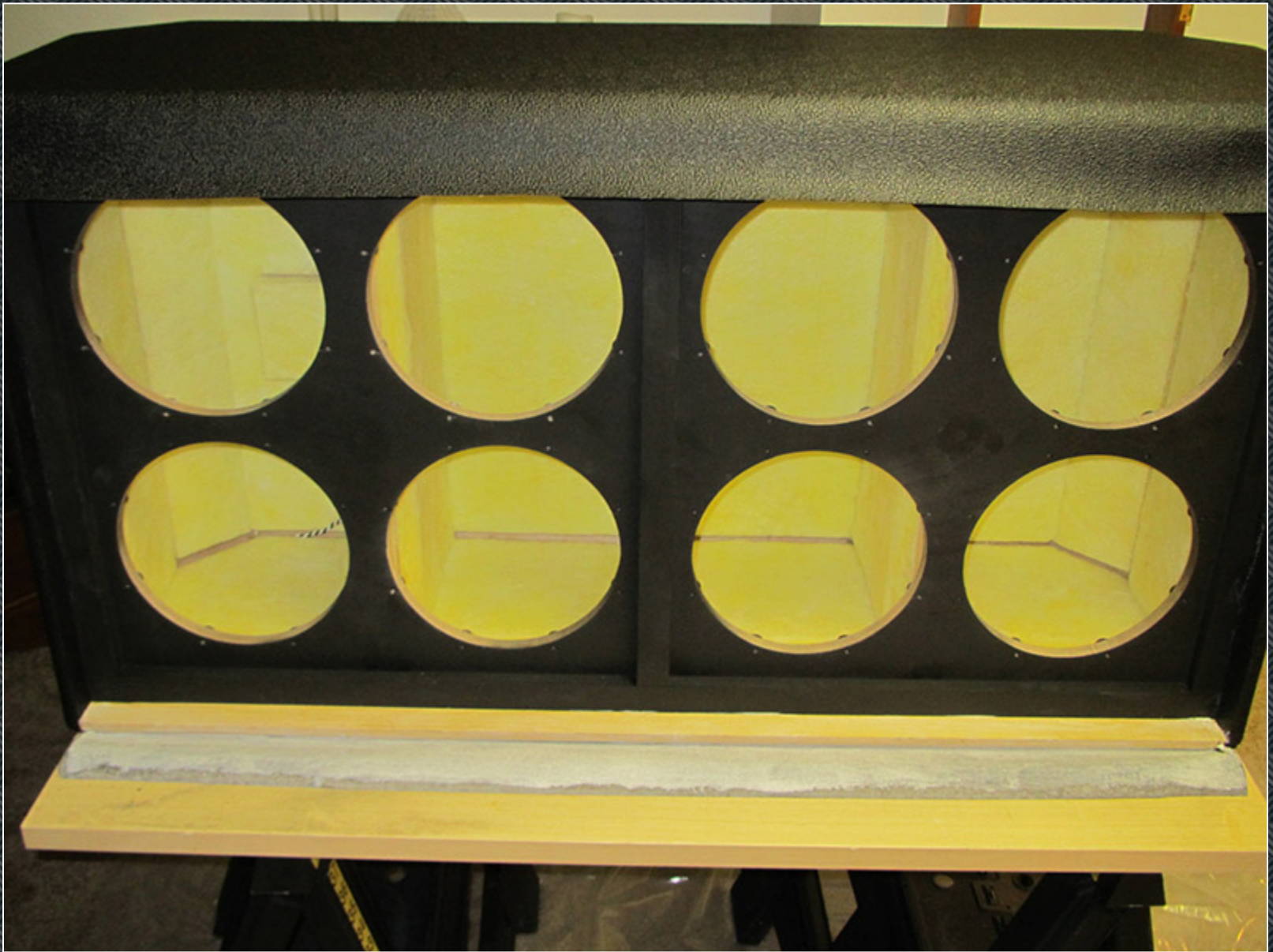
Gluing one of the side flaps.
