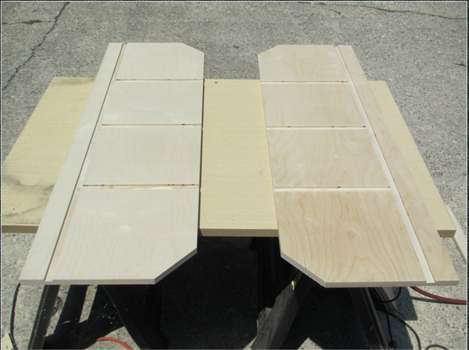
Here are the two sides with all the dados routed.
