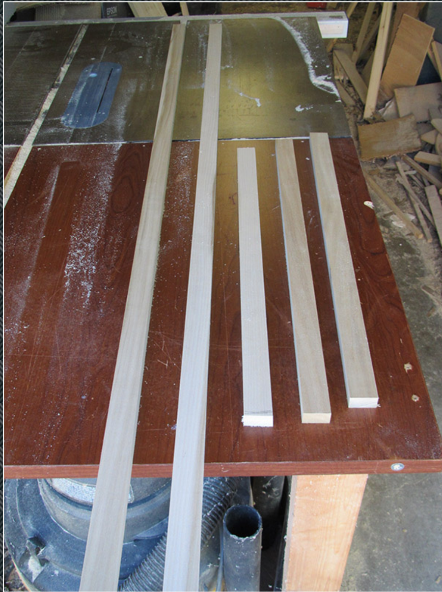
These are the 1-1/4" wide cleats that the grille frame will mount to.
