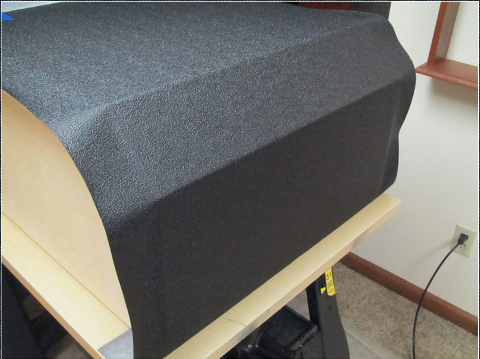
The Tolex glued down on the bottom.
