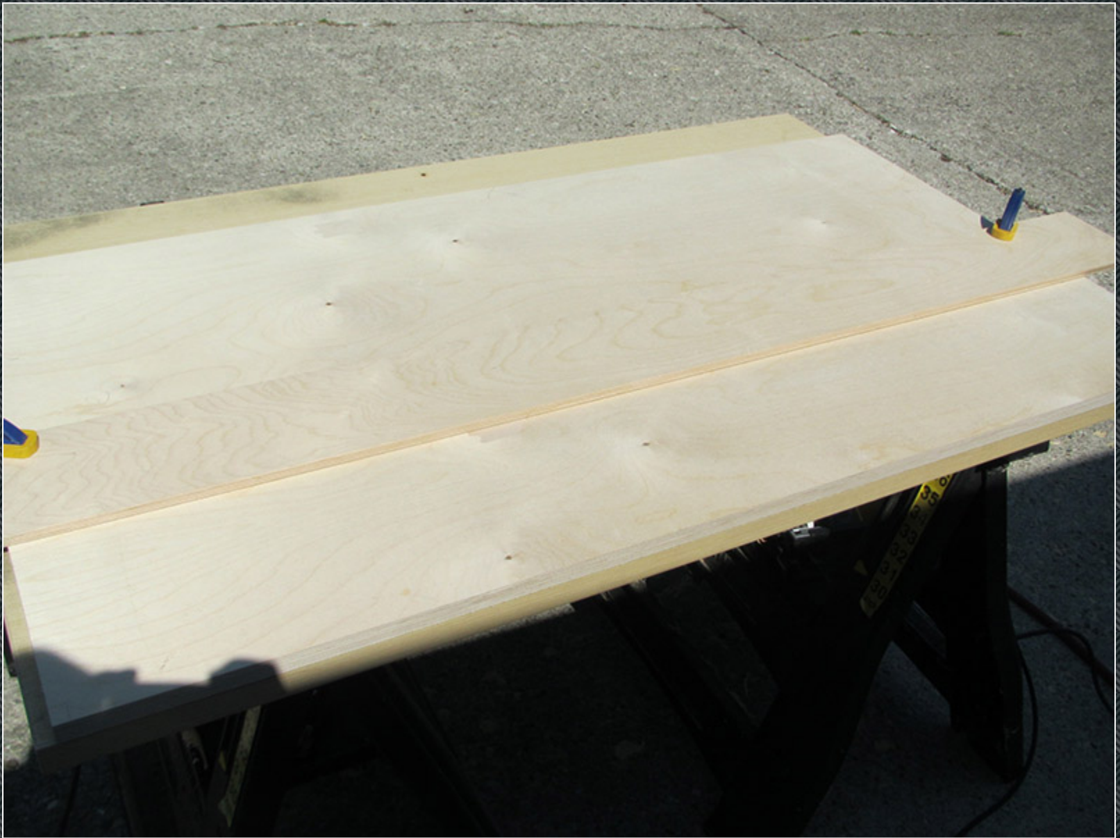
Starting to layout the centers of the speaker cutouts on the baffle.
