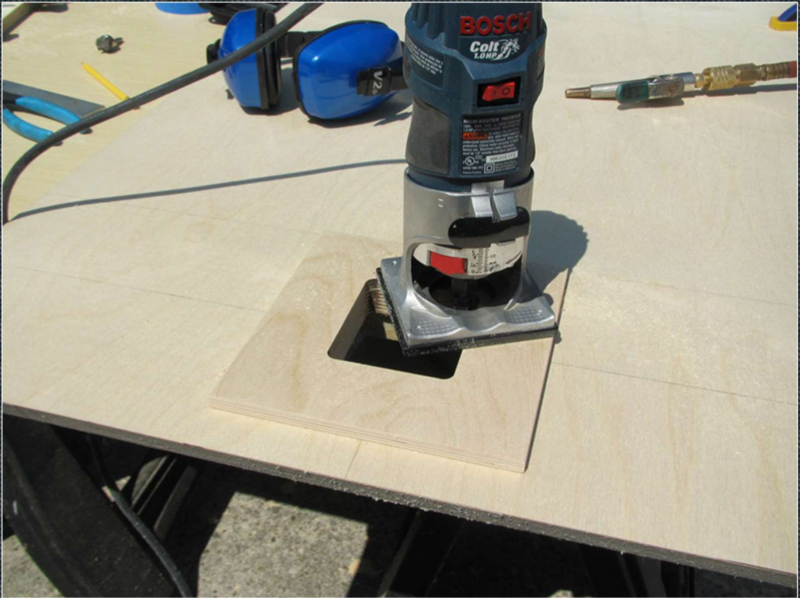
After attaching the template to the back with double face tape, I used the trim router and a template bit to clean up the cutout.
