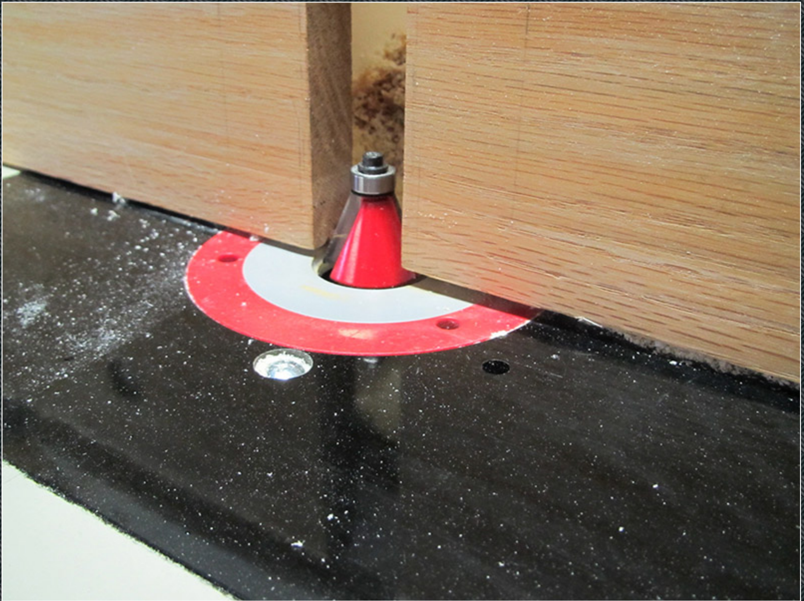
Router bit and fence adjusted to cut bevel.
