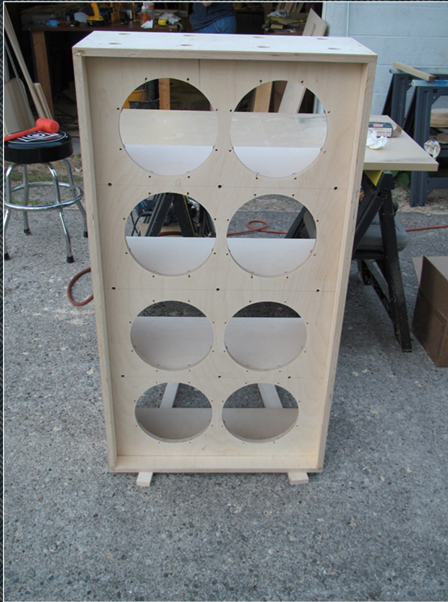
Front view of partially assembled cabinet (speaker baffle, sides, top, bottom, and dividers).
