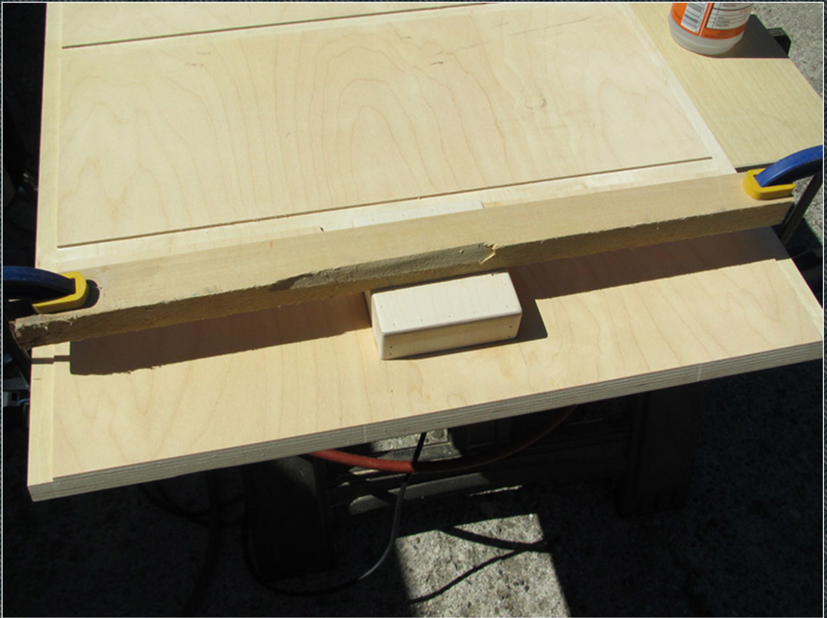
Box glued and clamped over the jack plate cutout in the back.
