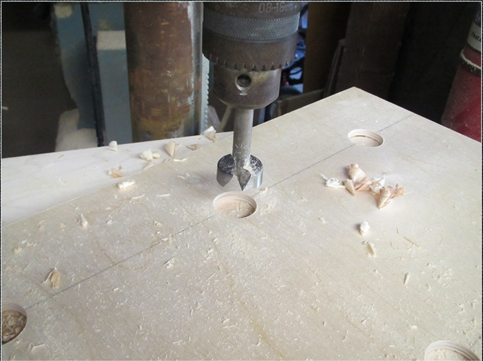
Drilling the foot cup holes using a 1-1/4" Forstner bit.
