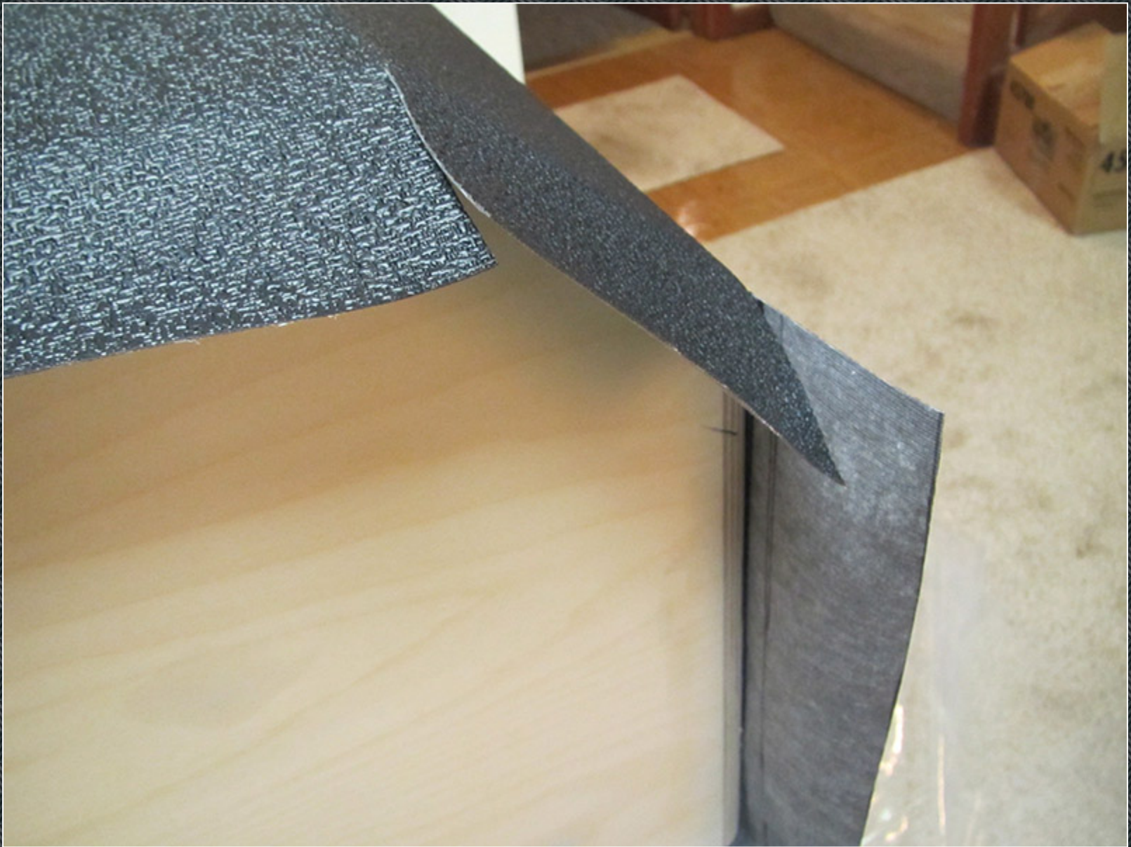
Cuts made to create flaps that will fold over the side.
