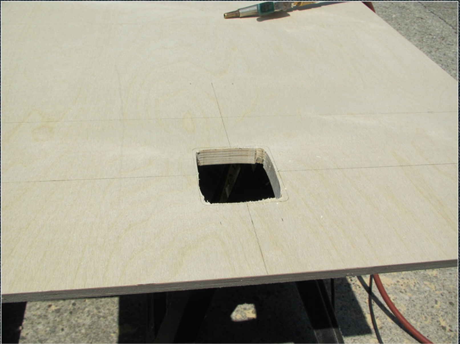
Here I have done a rough cut using the jig saw.
