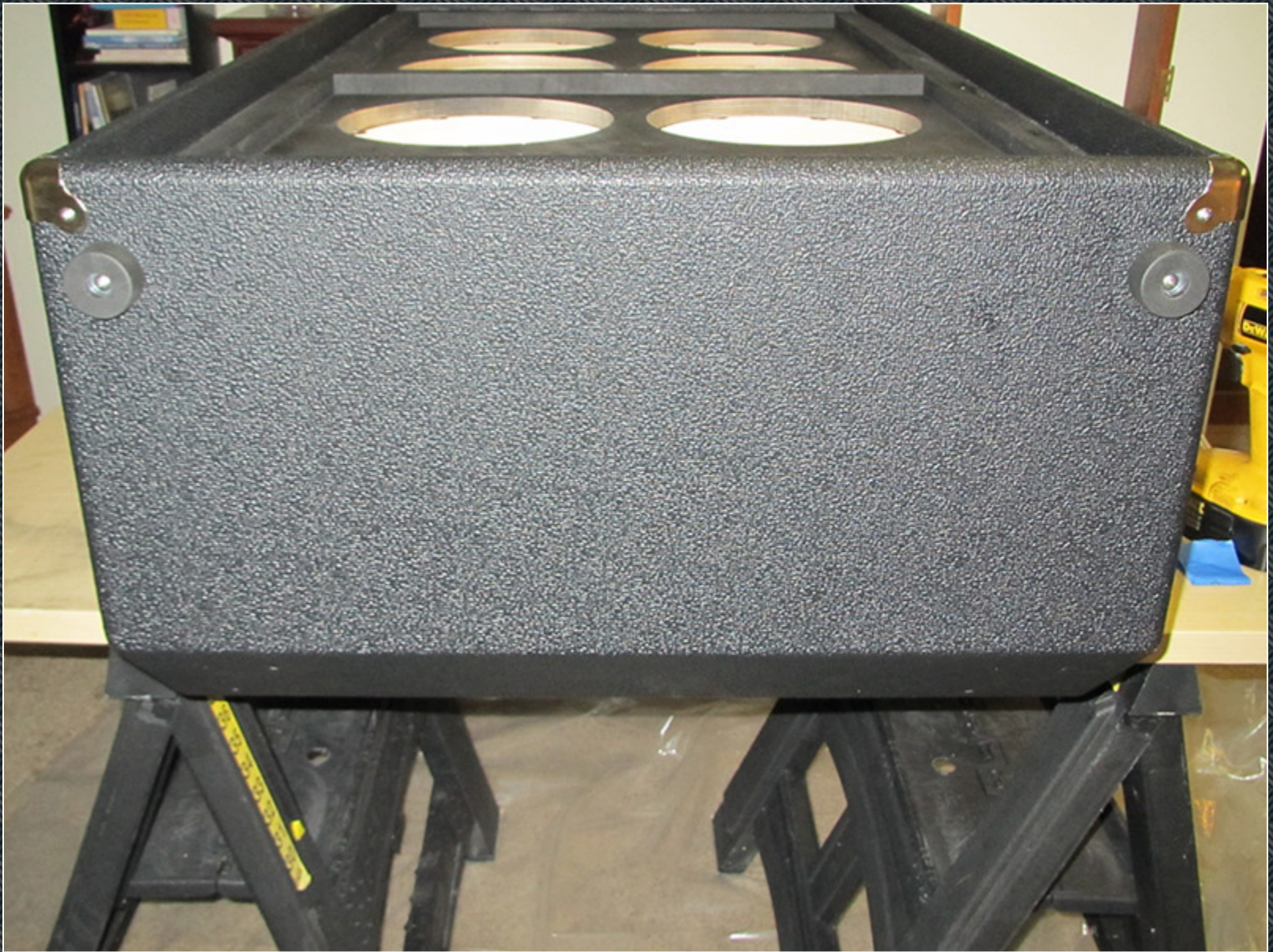
Both rubber feet installed.
