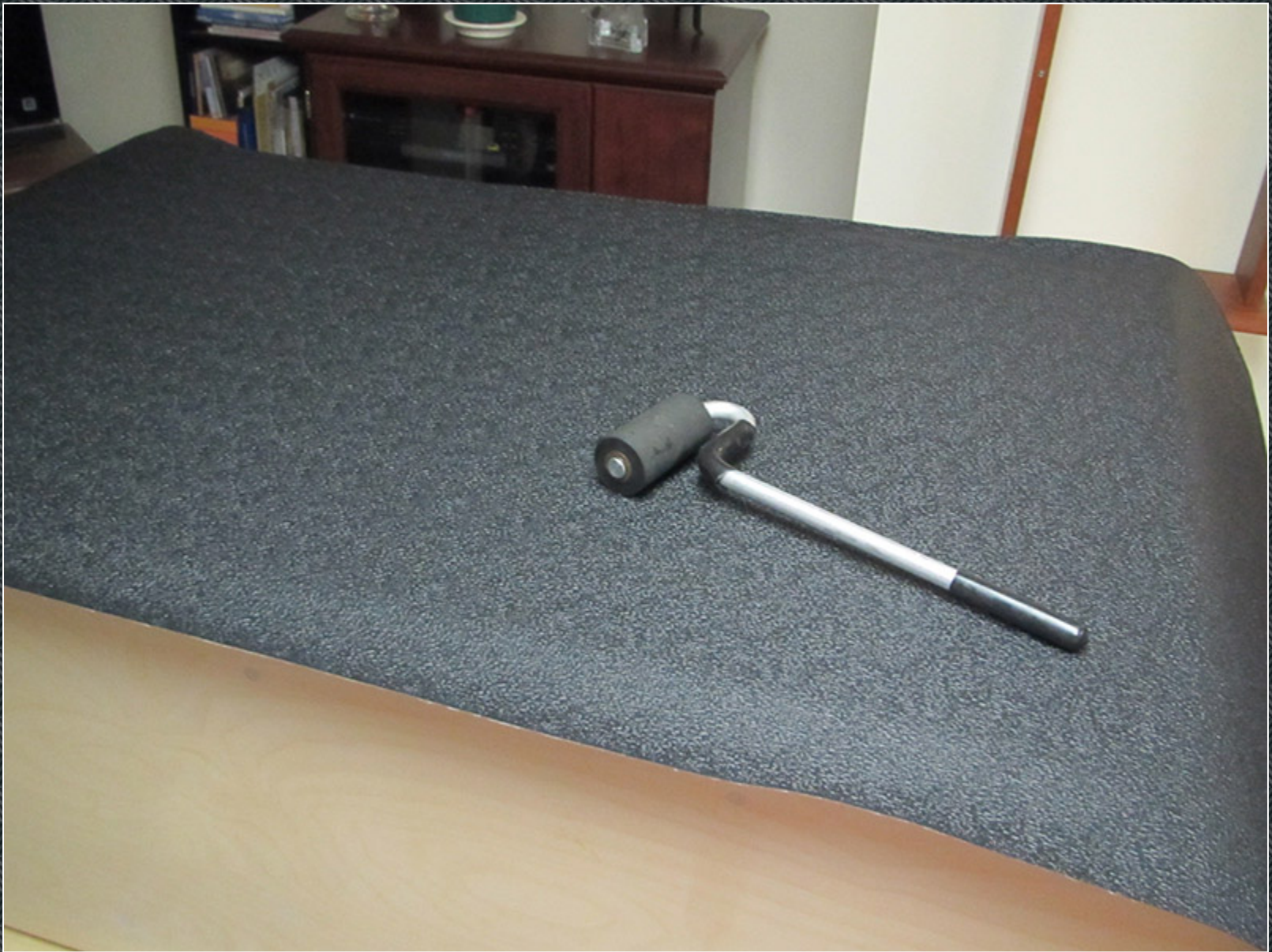
After lining the piece up and applying it to the back I used a J-roller to make sure it's flat and well-adhered.
