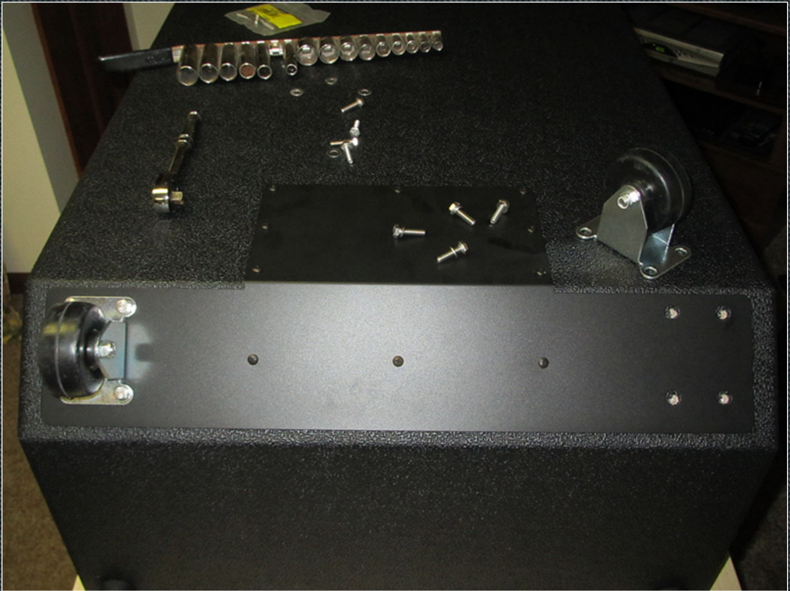
Installing the casters.
