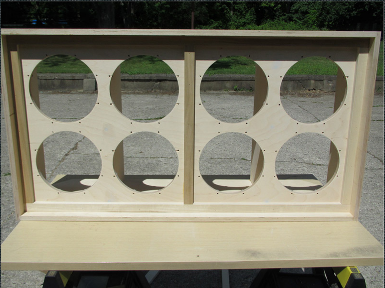
Cabinet with all of the cleats installed.
