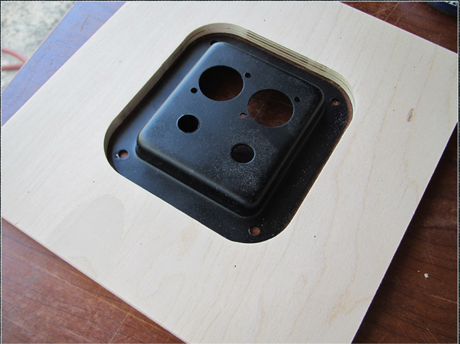
Using the jack plate to check the size of the template.
