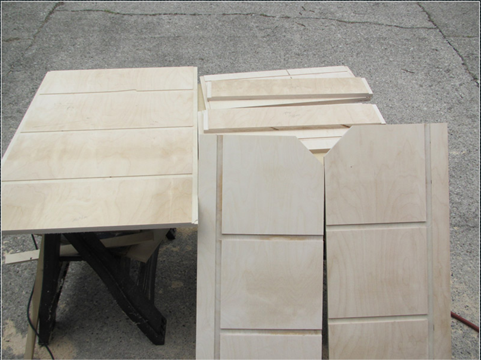
Here are all of the shell pieces cut to size, with all dadoes and rabbets routed.
