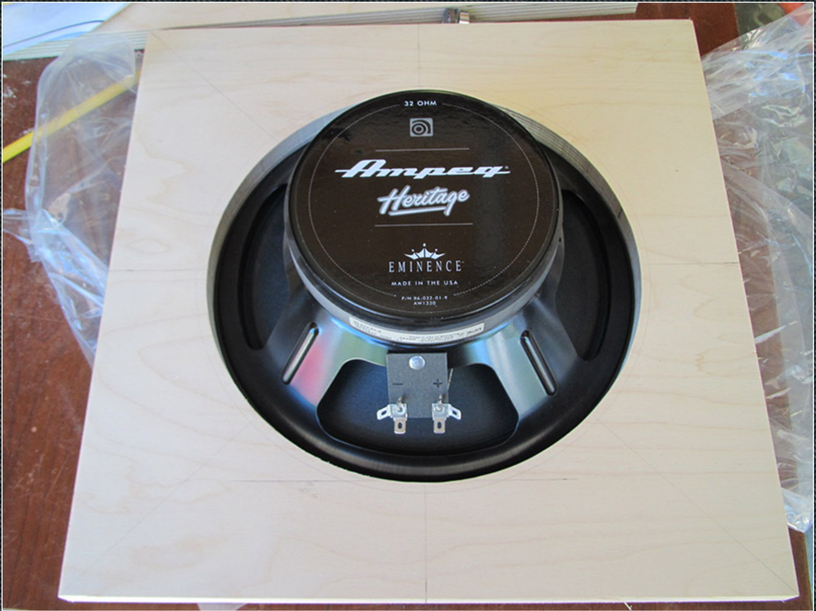
Checking the fit of my speaker cutout template with one of the speakers. The speaker was then used to locate and drill the mounting holes in the template.
