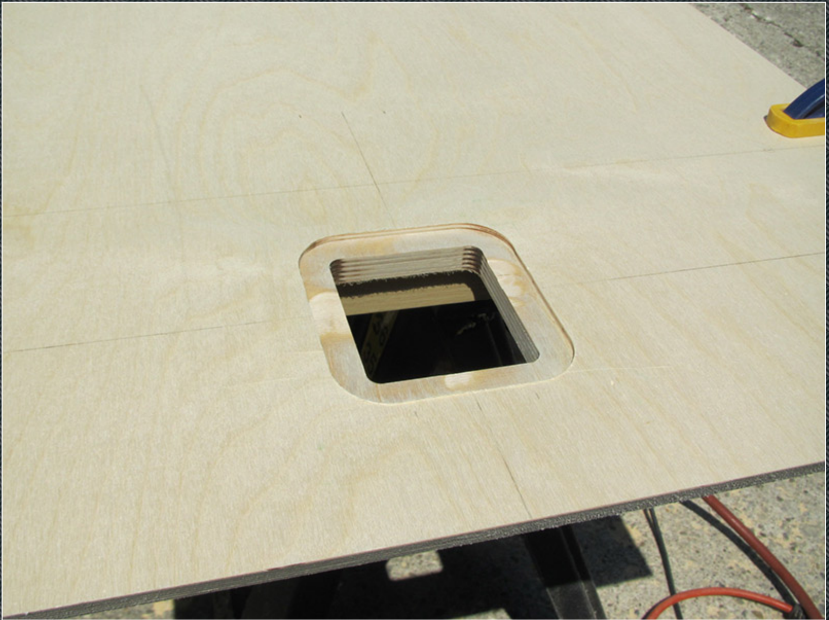
Finished jack plate cutout.
