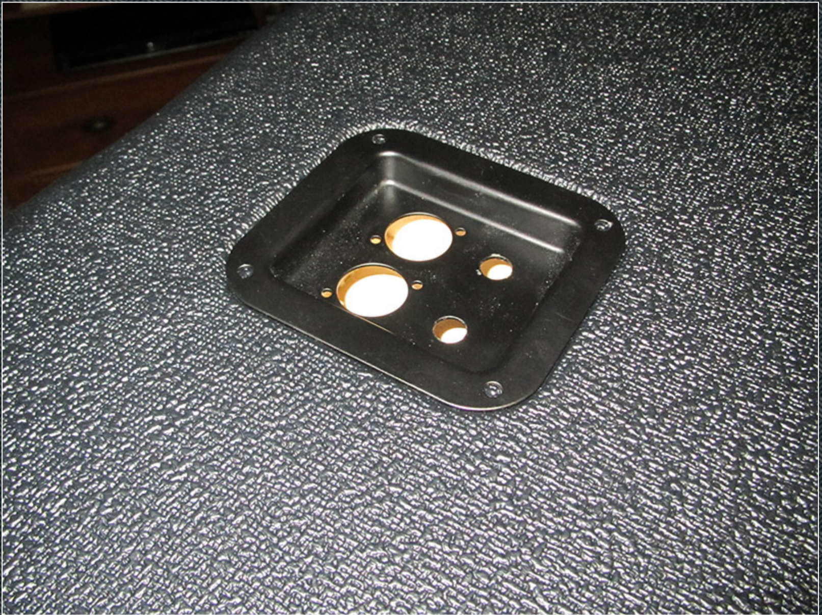
Laying the jack plate in to check the final fit.
