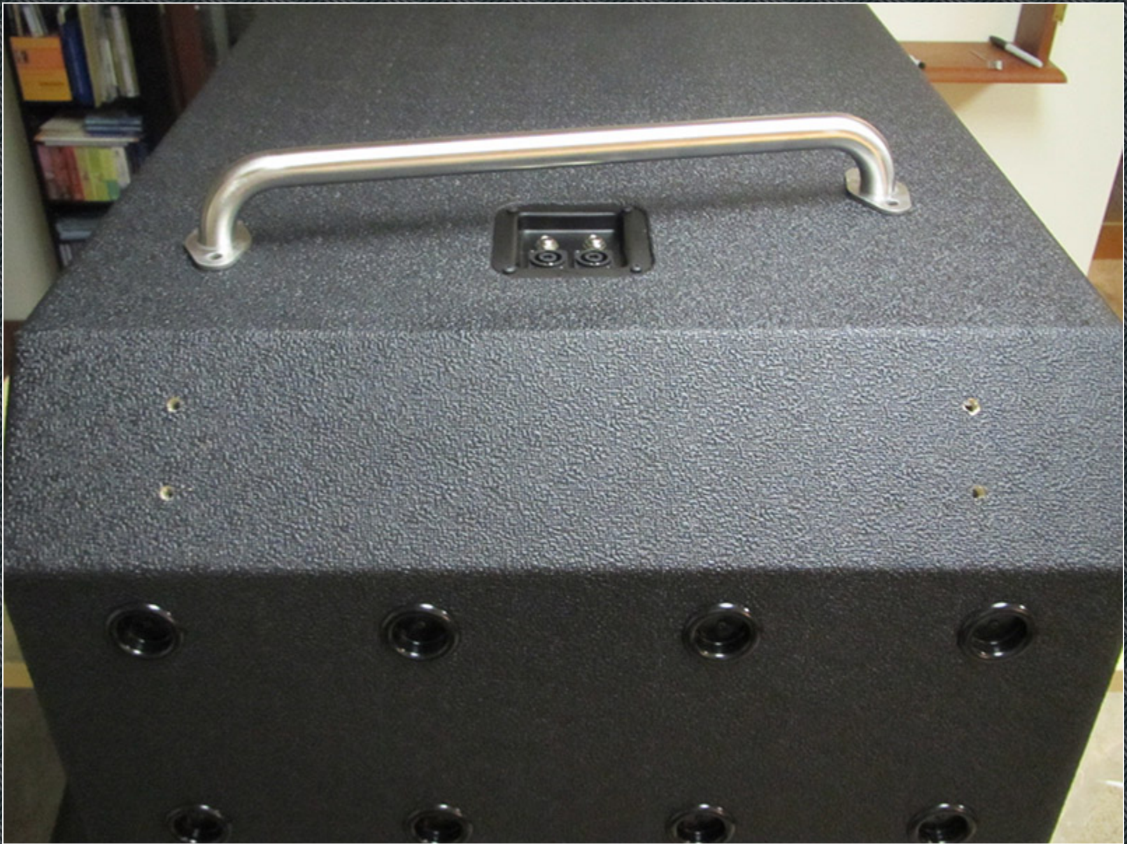
Drilling out the Tolex covering the towel bar mounting holes.
