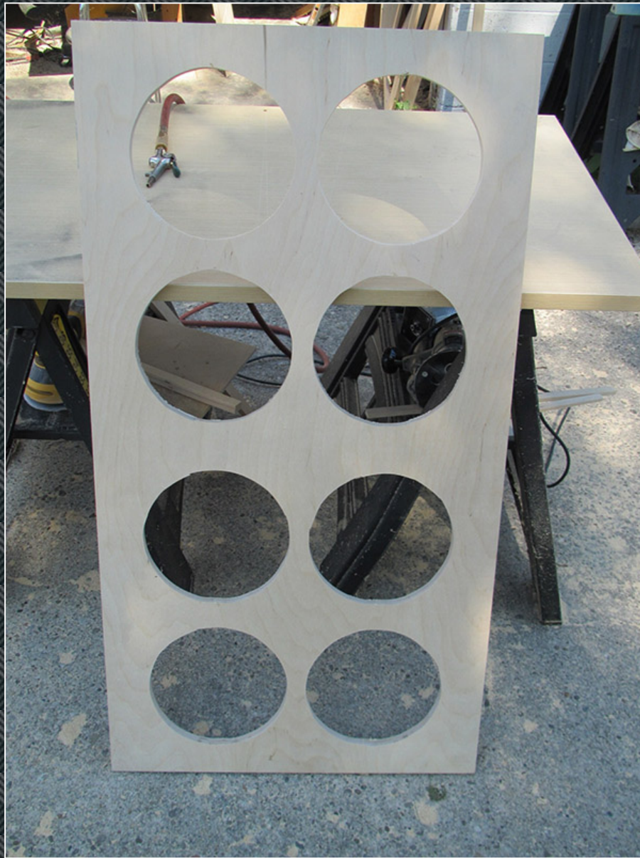
Speaker baffle after roughing out the cutouts with the jig saw.
