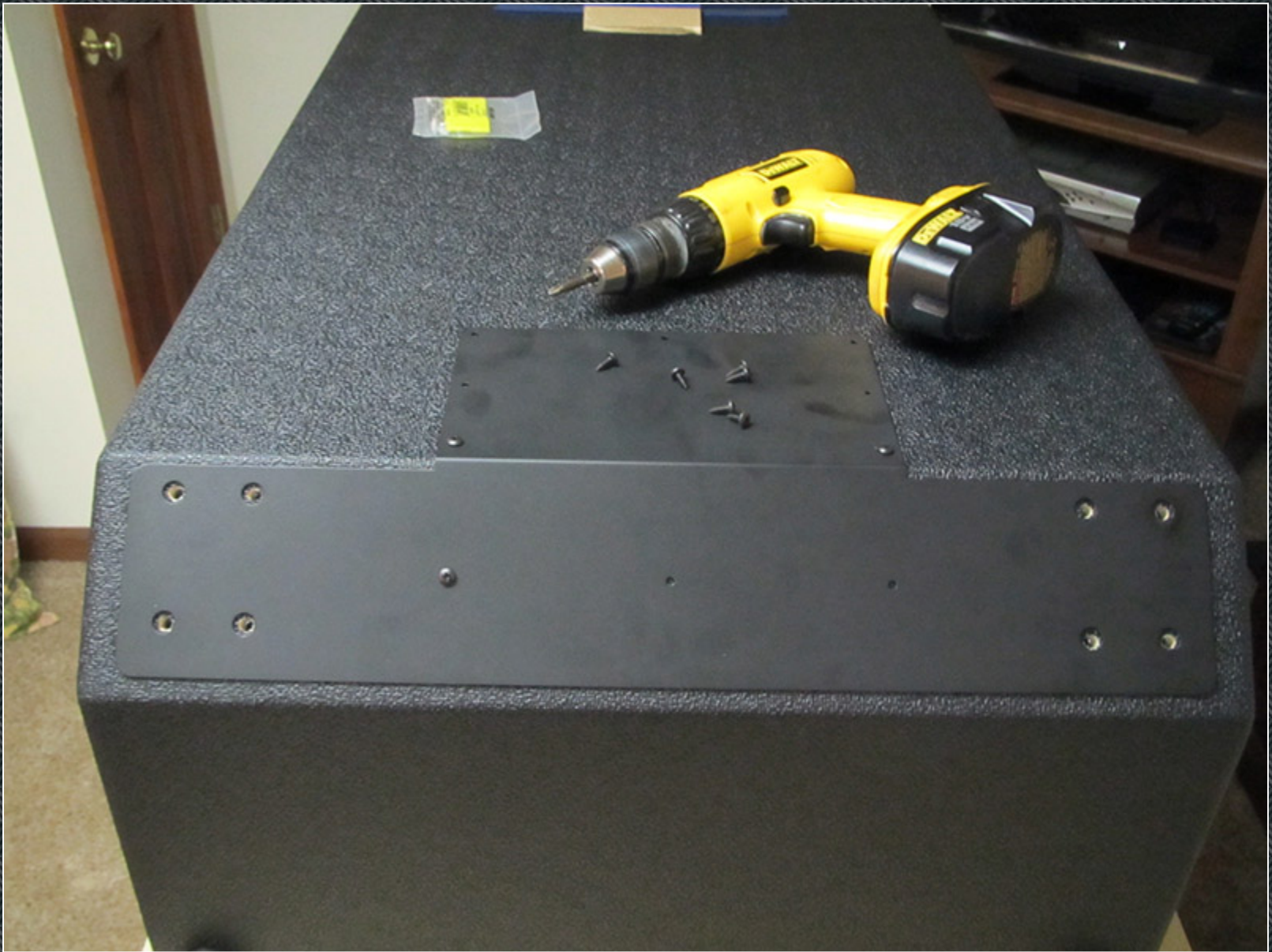
Installing the kick plate.
