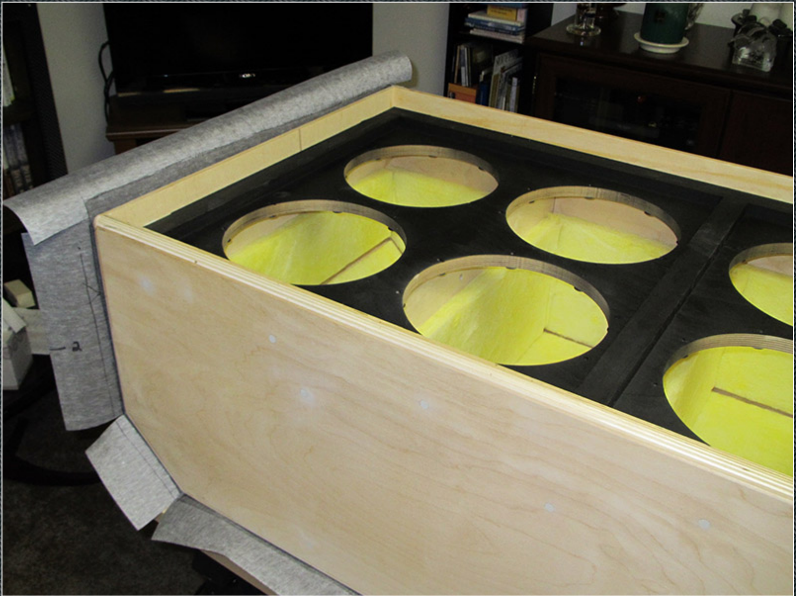
Preparing to fold the top flap over the top front of the cabinet.
