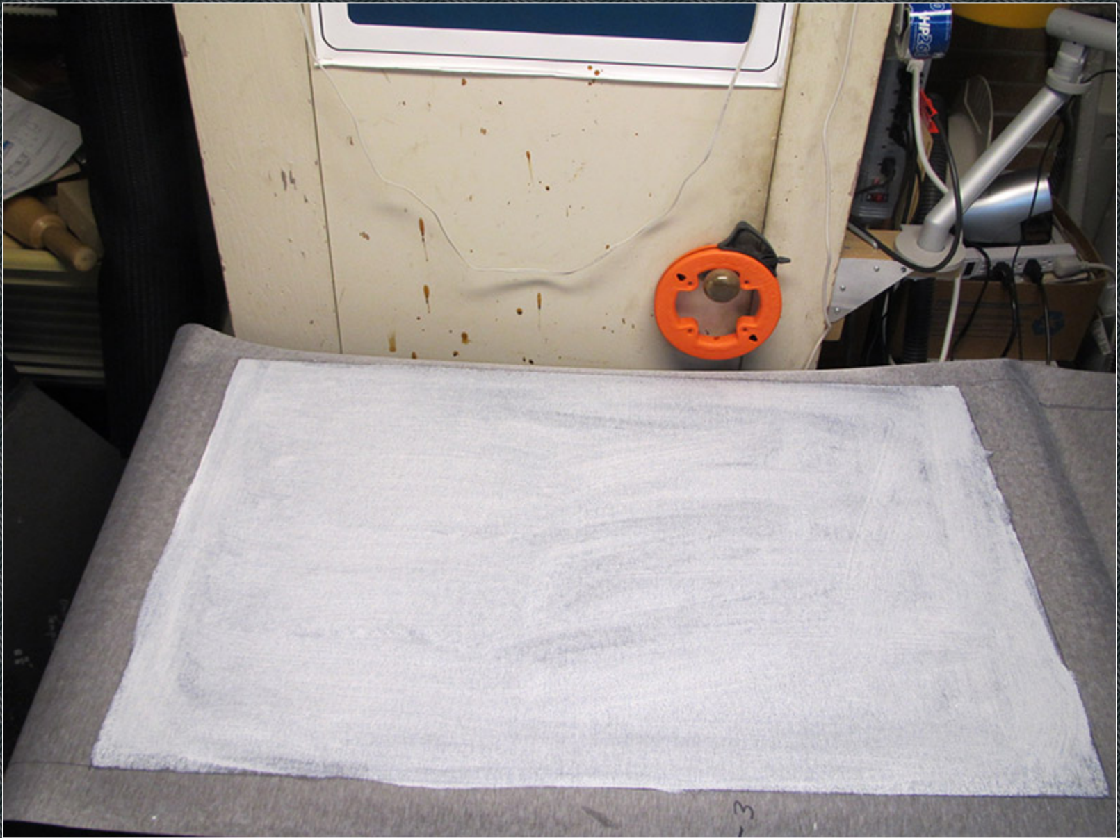
First glue application on the back. I am using a water-based contact adhesive.
