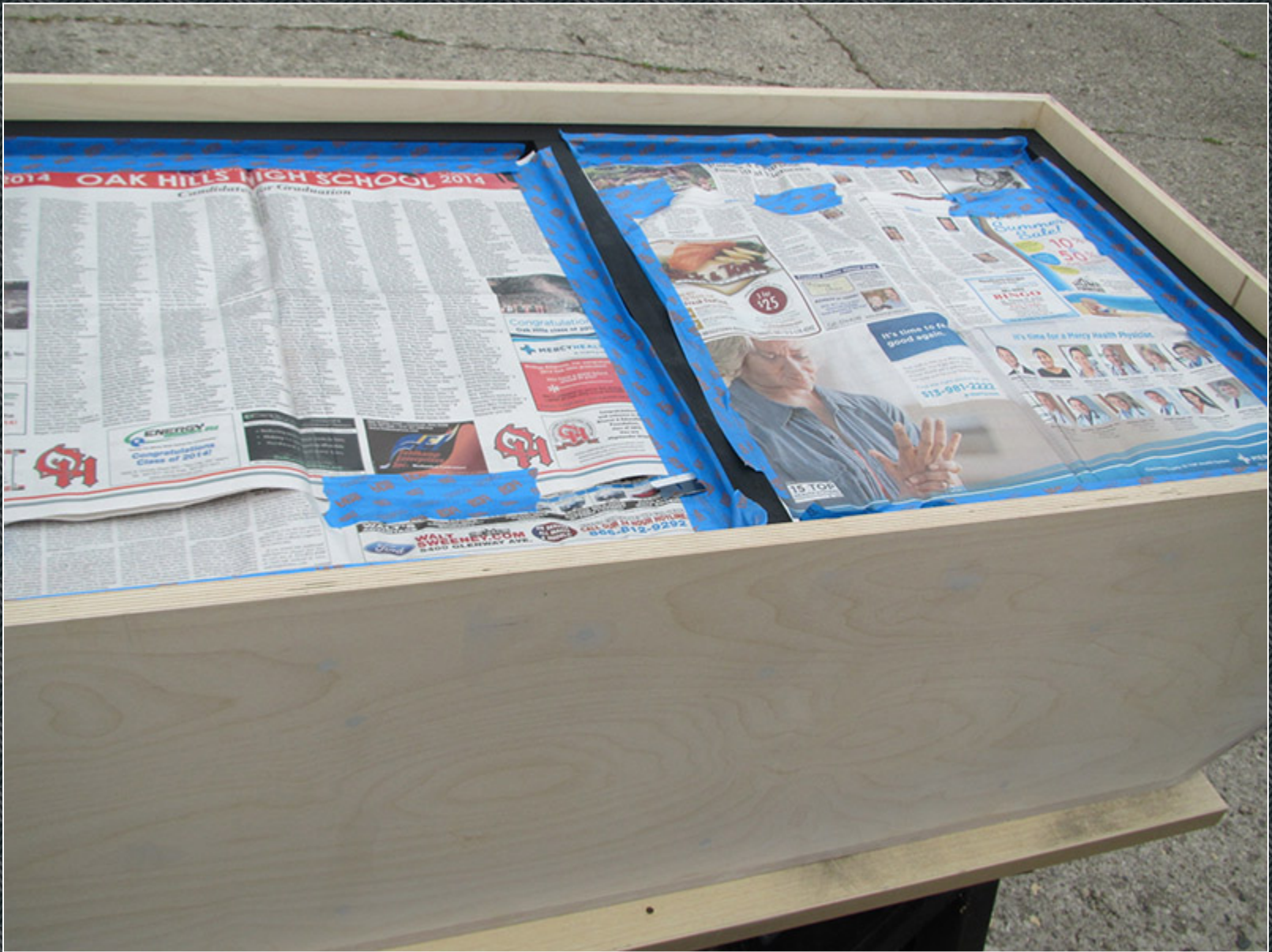
I was getting ready to rout the 1/2" round over on the cabinets edges and covered the speaker cutouts to help minimize any clean up later.
