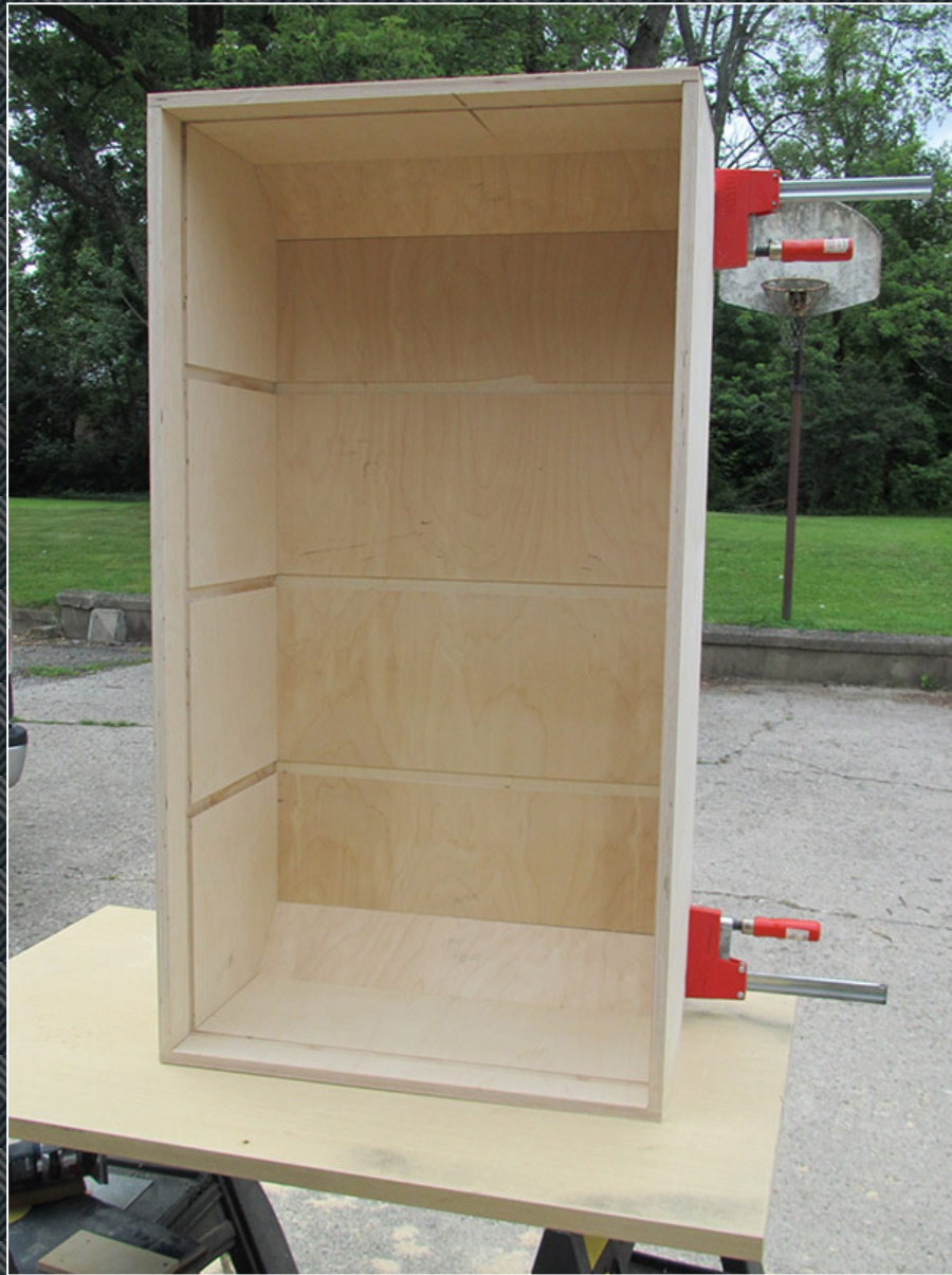
At this point I was able to do a dry fit to see how things were looking.
